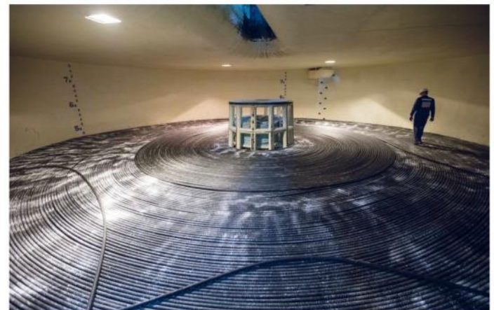
Big cable ships bunker thousands of kilometers of underwater cables. The cable is buried in flat water, simply cast off after it reaches a depth of 200 m
