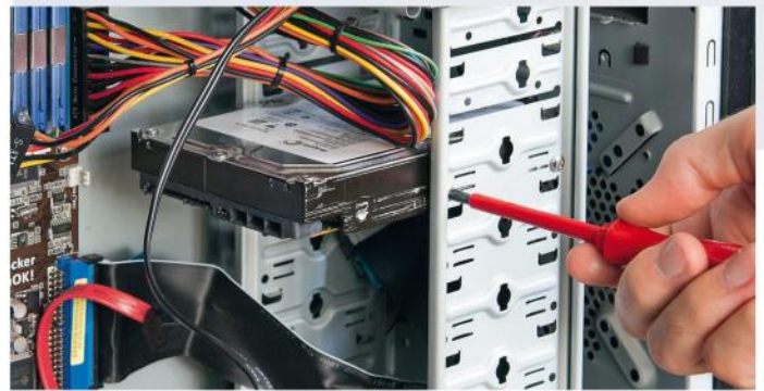
It's very easy to install an additional 3.5-inch SATA hard drive in a PC. Just screw it in tight, connect it, and you're done
