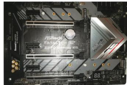
PCI-e Steel Slots add greater stability for heavier graphic cards
