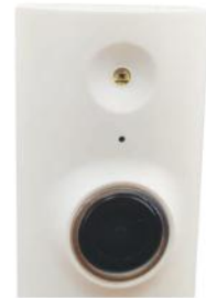
Seeing in the dark is no problem with the infrared sensor above the lens and microphone.
