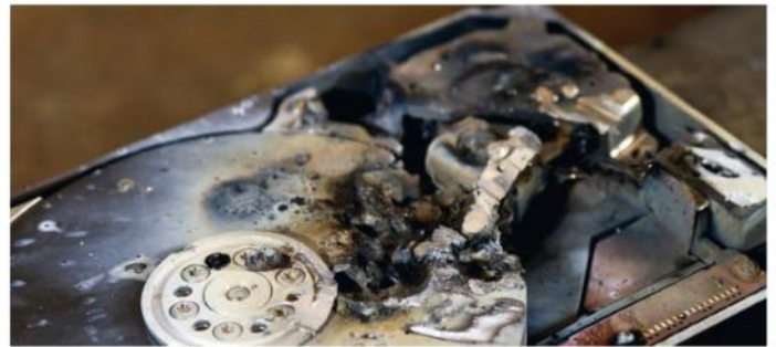
Sometimes even the professionals are powerless. Destroyed hardware (e.g. due to a fire) is a frequent and – above all – abruptly-occurring cause of data loss
